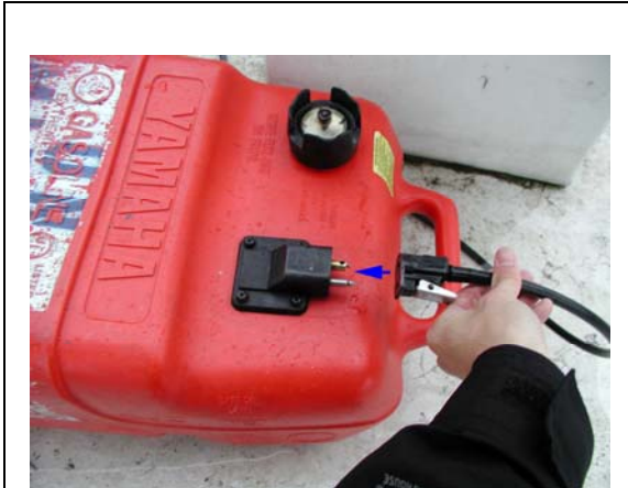
Figure 3: Connect the hose already in the Skiff to the unmixed gasoline container you brought with you.
